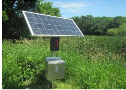
Figure 20. Solar panel mounted on pole to power Brandt PIT station
