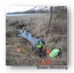
Flow measurements were collected by PLSLWD and Scott SWCD. Flow meters used include FloMate 2000 and a Sontek
