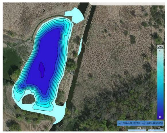
FIGURE 12 BATHYMETRIC MAP CREATED USING BIOBASE SOFTWARE AND PLATYPUS BOAT
