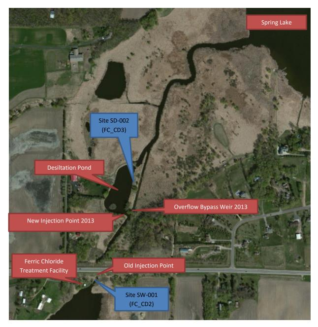
FIGURE 5 AERIAL MAP OF FERRIC CHLORIDE TREATMENT SYSTEM
