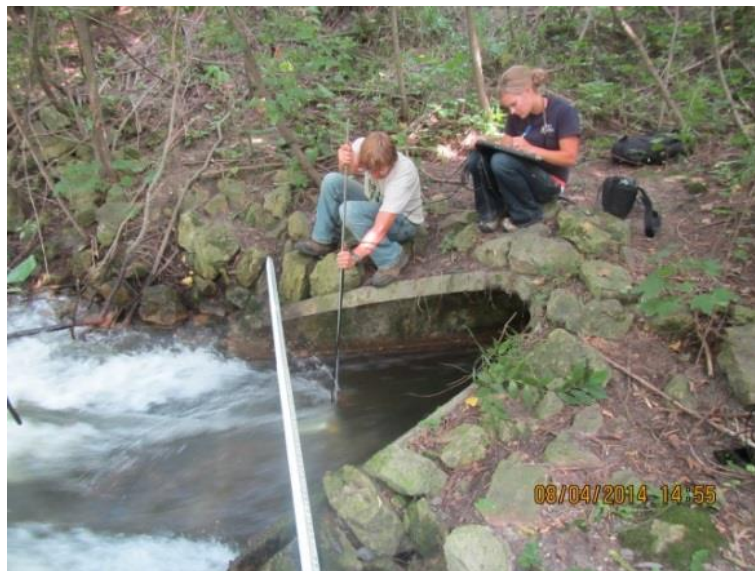
Figure 5 Water splashing on wading rod making it difficult to get accurate depth.
