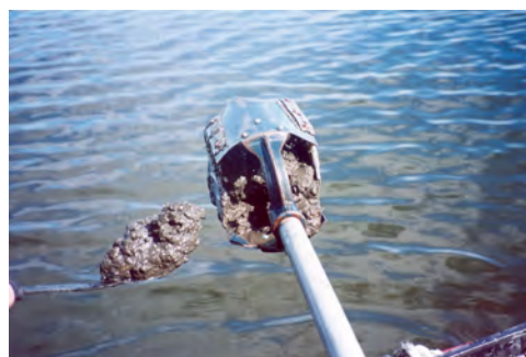
Figure 1. Soil auger used to collect lake sediments in shallow water.
