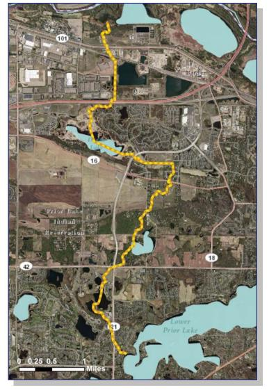
Map of the Prior Lake Outlet Channel (PLOC). The PLOC receives water from Lower Prior Lake and the surrounding watershed and discharges into the Minnesota River.
