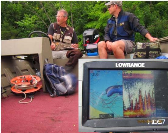
BioBase uses sonar to detect and record aquatic vegetation density, lake bottom hardness, and bathymetry (contours of lake bottom). Vegetation density is determined by the percent of the water column (the vertical space between the lake bottom and the water surface) that is filled with plants. An area that has plant growth from the lake bottom to the lake surface has 100% vegetation density, while an area of the lake with no vegetation has 0% density.
